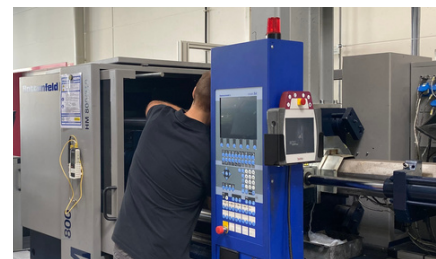
Installing the tools
