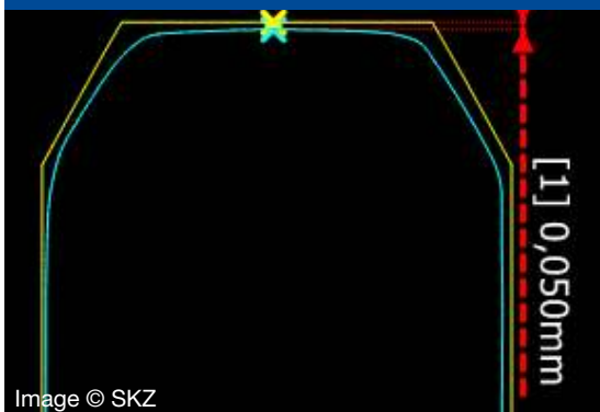
Profile comparison (2D) of a pin in a tool (turquoise) and its .stl (yellow)
