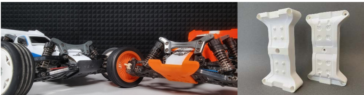
Bumpers made from PA (black) and PP GF30 (orange) on the left; the associated two-cavity mold (right). Images © DREIGEIST
