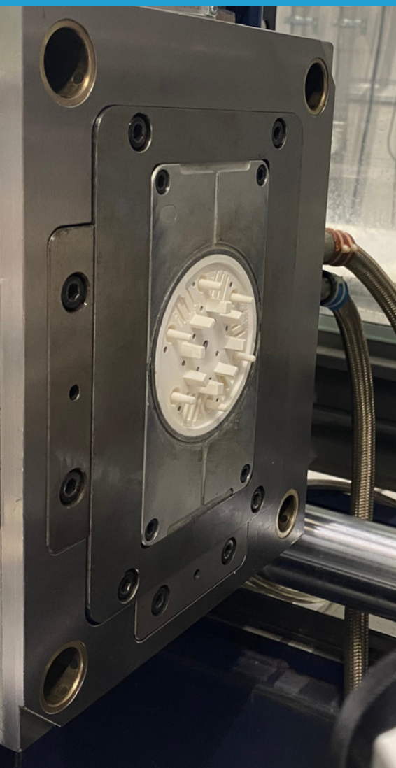
3D printed tool insert Image © DREIGEIST
